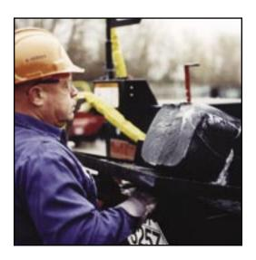
Low loading heights and loading doors positioned above the fenders of the model supply correct ergonomics, preventing repeated stress and lifting injuries. A properly designed angled loading door, when closed quickly, prevents splashing of hot sealant.
