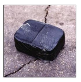
This particular hot melt crack and joint sealant block is the equivalent of 3 gallons of melted sealant. The block weighs approximately 30 pounds, equaling 10 pounds per gallon.
